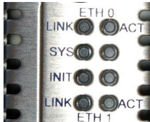
Figure 15: Diagnostic LEDs (Front View).
